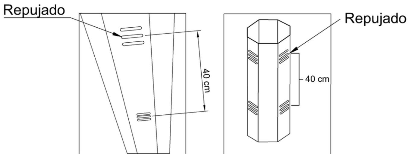
FIGURA 2.A DETALLE DEL REPUJADO
