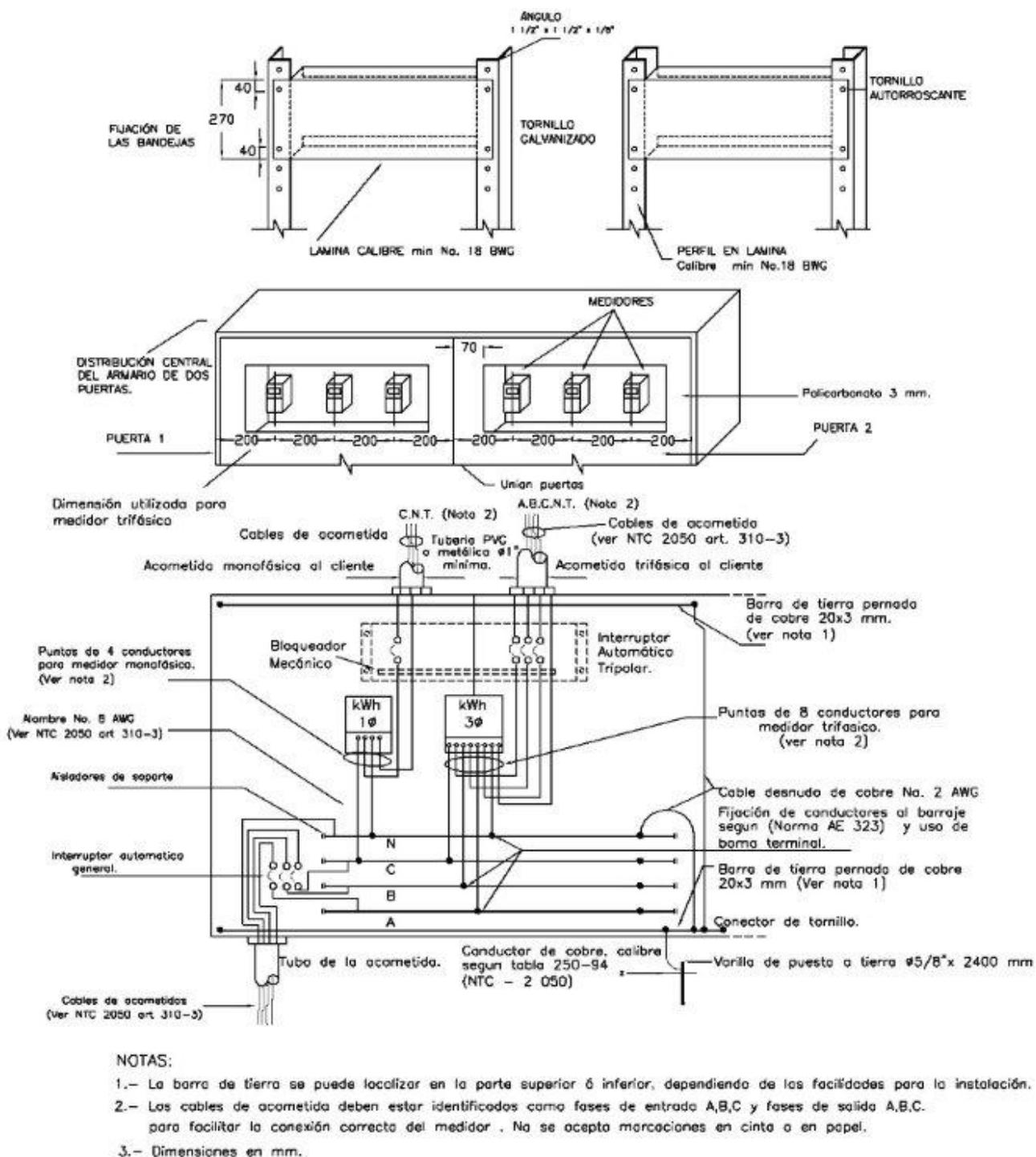
**FIGURA 6. ARMARIO CON TOTALIZADOR Y BARRAJE LATERAL**
