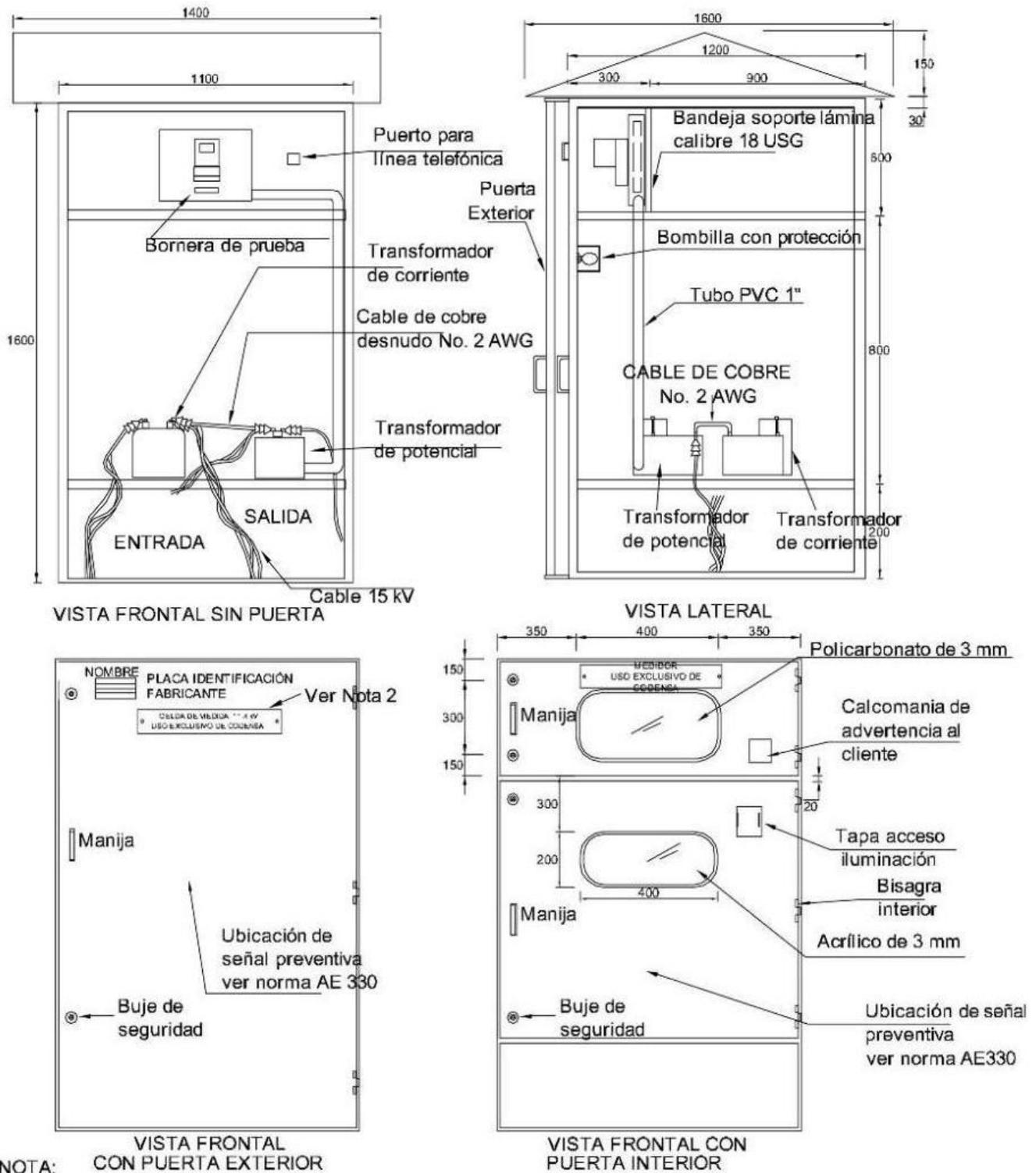
**FIGURA 8. CELDA DE MEDIDA 34,5kV TIPO INTEMPERIE**
