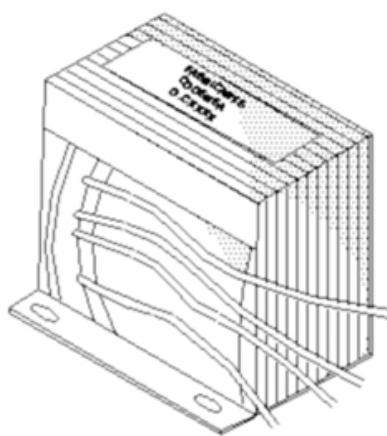
A Balasto Reactor
